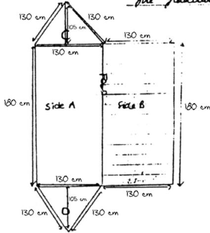
Side A and Side B are the two sides and fold over to each side of triangles C and D which are the doors
