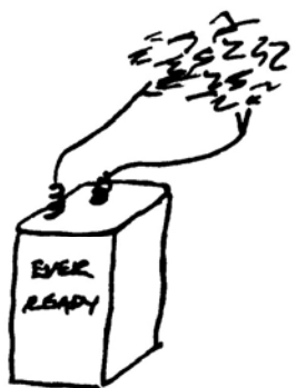
Fig A4.1: Diagram showing how battery should be connected to steel wool.
